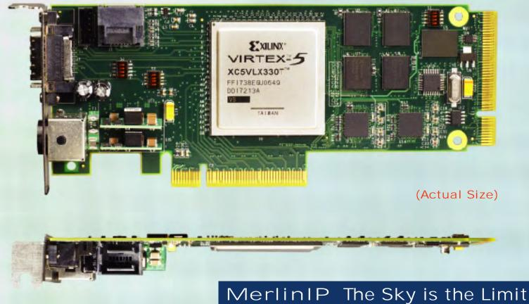
The MerlinIP is designed to support your most challenging projects. Small, fast, and customizable, the MerlinIP sets a new standard for an Audio/Video hosting platform. Featuring the powerful Xilinx<sup>TM</sup>Virtex<sup>TM</sup>-5 FPGA, the MerlinIP provides unparalleled IP Core integration and development possibilities with scalable Virtex-5™ models and pricing, giving you just the capacity you need.
